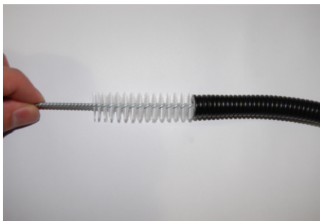
Fig. 66: Clean pump hoses
