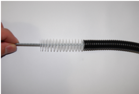
Fig. 39: Clean pump hoses
