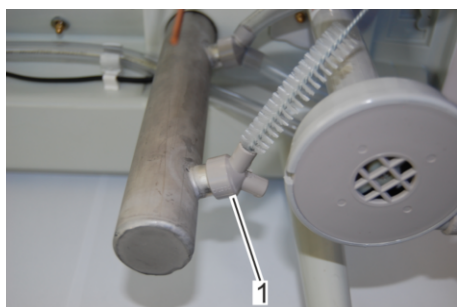
Fig. 67: Cleaning the stainless steel pipe
