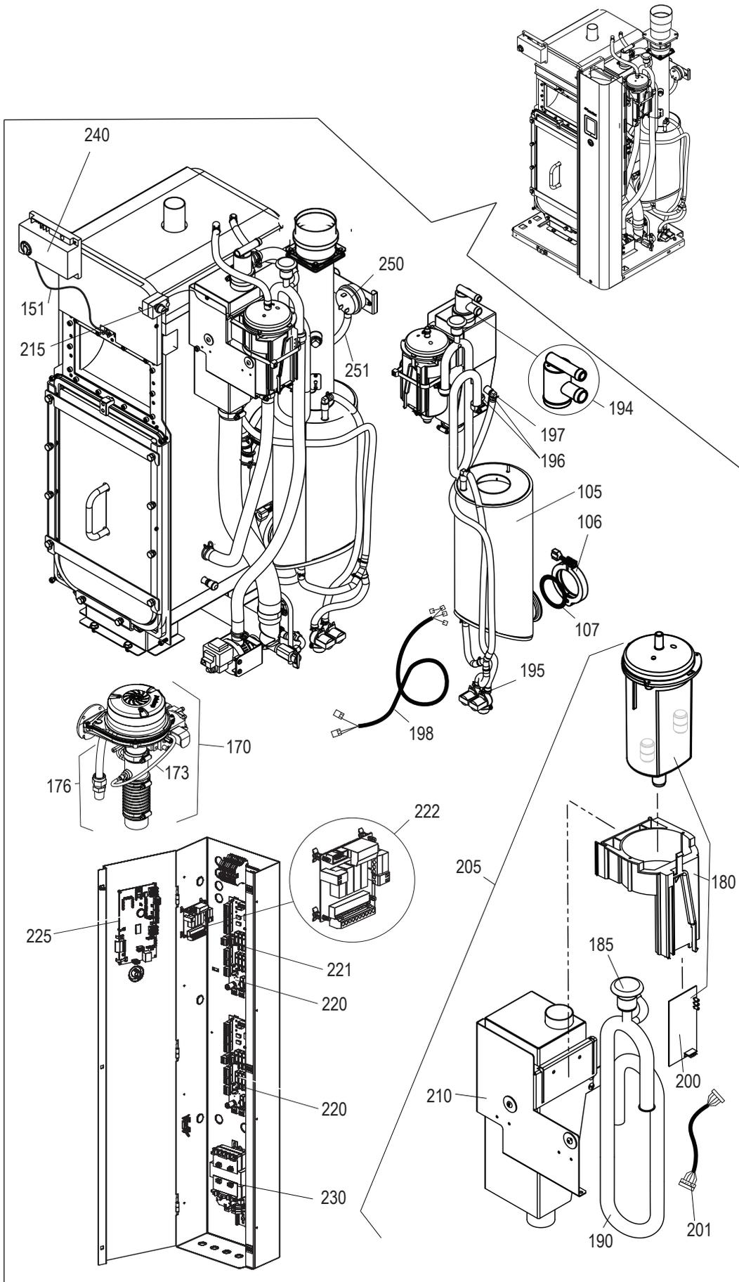
Figure 2: Nortec GS 100 Humidifier, Plumbing and Electrical. .
