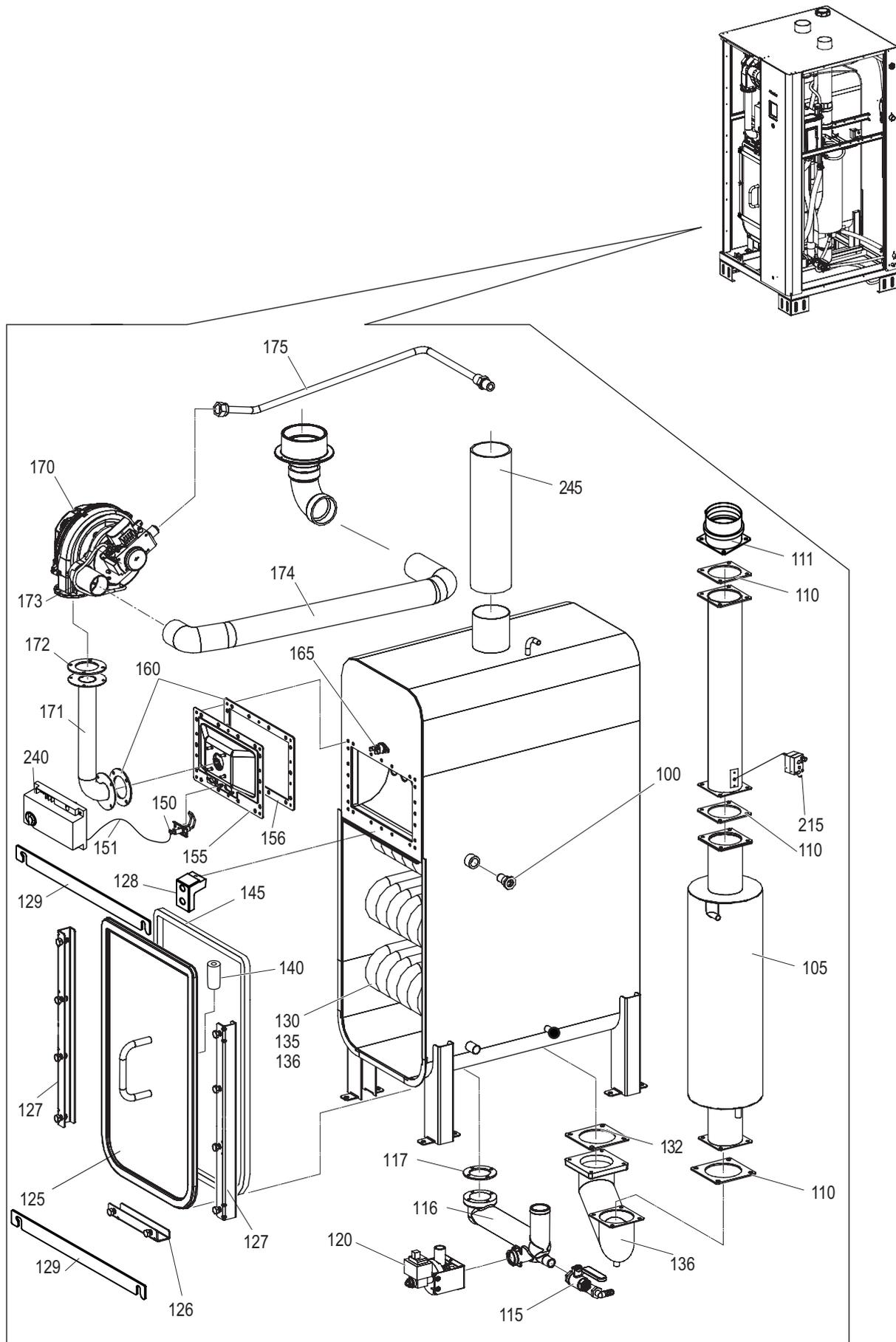
Figure 1: Nortec GS 150 Humidifier, Heat-exchanger and Blower
