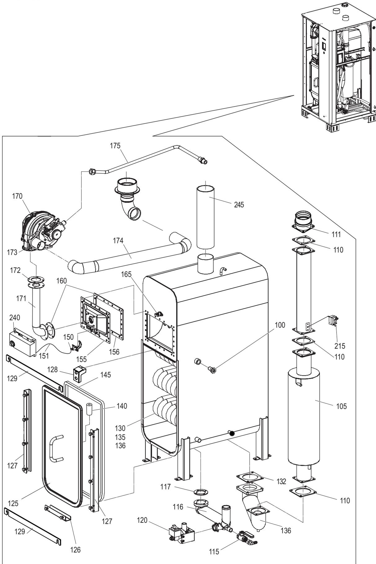
Figure 1: Nortec GS 150 Humidifier, Heat-exchanger and Blower, continued...
