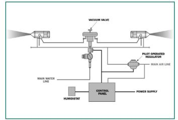
mounted with spray from one side (single configuration) using 3 or 4 AFE nozzles. AFE OCTO systems are available with or without a AFE control panel built into the case. AFE OCTO systems are available for use with normal tap water, reverse osmosis, or deionized (DI) water.
