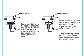
Figure 7 Vacuum Valve and Interfaces
