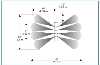
Figure 16 Four OCTO Systems Operated From One Control Panel, is a typical installation layout for 4 OCTO units and a control panel. The pilot air pressure input to the control panel is connected directly to the air pressure line (90 psig) (621 kPa) by 1/4 inch plastic tubing. The "Pilot - Out" from the Control Panel is the command pressure which can be
