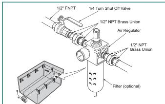
It includes a shut off valve, primary air regulator (0 to 100 psig) (0-690 kPa) and a pressure gauge, and a filter (optional). It is threaded to connect with  $\frac{1}{2}$ " NPT female thread. See page 12 for component specifications.
