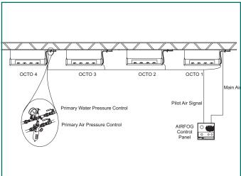
"T" connected to all four OCTO systems. In this way, one Control Panel can control up to 4 OCTO systems.
